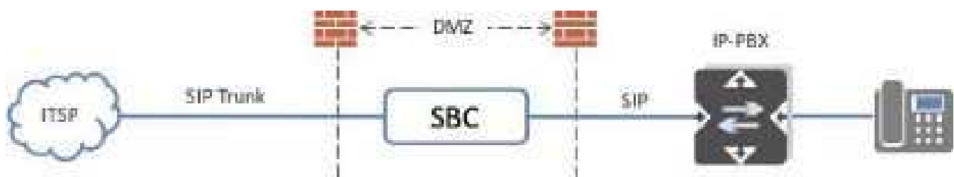
Enterprise SIP Trunking
