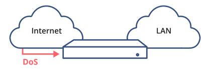
Rate Limiting on SIP methods is to determine the number of INVITEs or new calls (or other SIP methods) that the SBC is going to allow to traverse through to the VoIP servers. This is beneficial when wanting to restrict the number of new calls presented in a given period of time.
