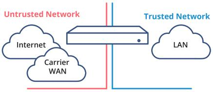
It is important to place an SBC between trusted and untrusted IP networks to provide security policies and ensure that each network does not have a direct connection. The Internet is the most untrusted IP network, and carrier private WAN IP networks are also outside the security of the enterprise trusted LAN network.
